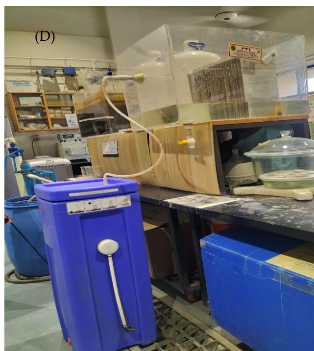
Figure 1. Schematic and digital image of the combined ECF system: (A) raw feeding tank with the capacity to store 200 L; (B) EC unit consisting of the EC electrodes inside a water tank with a volume of 200 L; (C) PAUL filtration unit; and (D) digital image of the complete pilot ECF system with Fe and Al electrodes EC units and PAUL filters.
