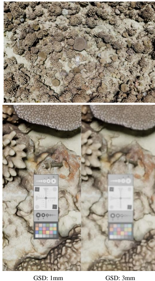
Figure 7. 3D model of a coral reef plot in Moorea, French Polynesia, used in POSER to interactively teach underwater photogrammetry fundamentals such as GSD, overlap, and side lap.
