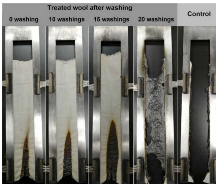
Figure 19. Results of vertical flame spread tests performed on wool fabrics treated with ammonium phytate (dry add-on: 14.2 wt.%) before and after laundry cycles. Reprinted with permission from [98]. Copyright Elsevier, 2022.
