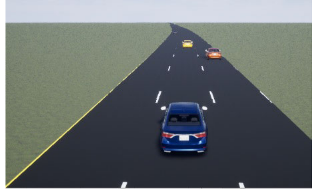
FIGURE 14. Vehicle positions during the second section of the simulation. The HV (blue) overtakes the orange car in the first lane. On the third lane, the distance from the purple vehicle is enough to begin the second overtaking maneuver of the yellow car.
