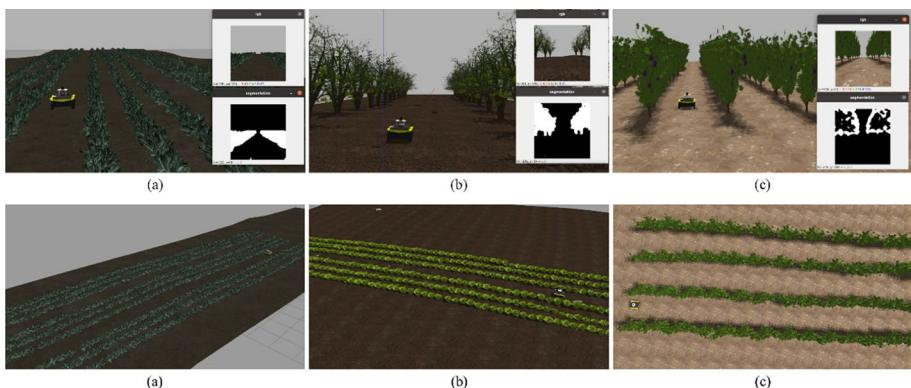
**Fig. 9** Validation of segmentation-based control of the robotic platform in the realized simulated environments. The upper row shows the Jackal UGV in chard (a), pear trees (b) and vineyard (c) fields in Gazebo from the robot perspective and current image with the predicted segmentation mask. The bottom row show UGV in chard (a), lettuce (b) and vineyard (c) fields in Gazebo from above
