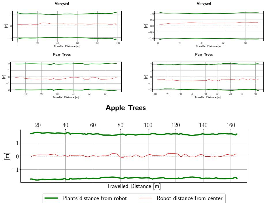
**Fig. 10** Trajectories performed by the real robot in rows of vineyard, pear and apple trees. Segmentation-based visual control proves to be an effective solution to counteract small obstacles and terrain deviation from the central path
