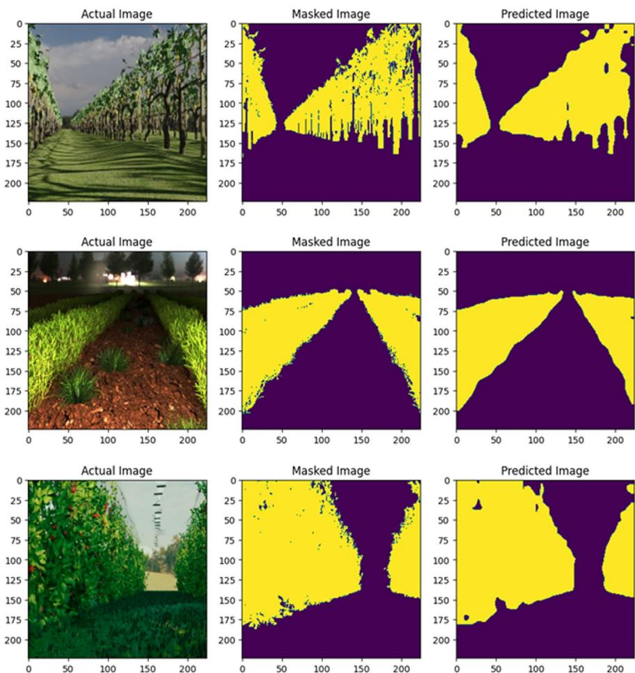
**Fig. 7** Test of semantic segmentation DNN on synthetic test samples from vineyard (top), lavender (middle) and apple trees (bottom) fields. For each crop, RGB input image (left), ground truth mask (center) and the predicted mask (right) are reported
