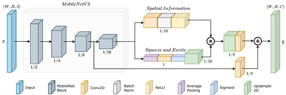
**Fig. 6** The Deep Neural Network used for the study. It presents a MobileNetV3 backbone and LR-ASPP head (Howard et al., 2019). Below each block, spatial scaling factor of the features compared to the input size is reported
