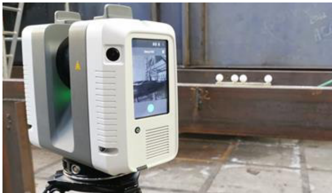
Fig. 2. Leica RTC360 wireless laser scanner used for conformity verifications at a Fincantieri S.p.A. shipyard.
