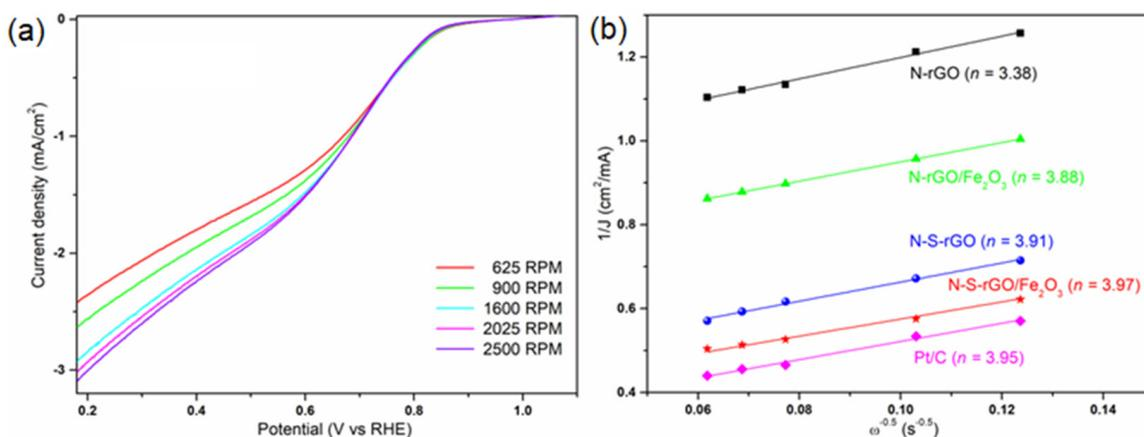
**Figure 7.** The results of the RDE measurements in a 0.1 M KOH solution: (a) ORR polarization curves of the N-S-rGO/Fe<sub>2</sub>O<sub>3</sub> sample at different rotation speeds; (b) Koutecky–Levich plots of the different catalysts at a 0.38 V potential (the numbers between parentheses represent the calculated electron transfer number values).
