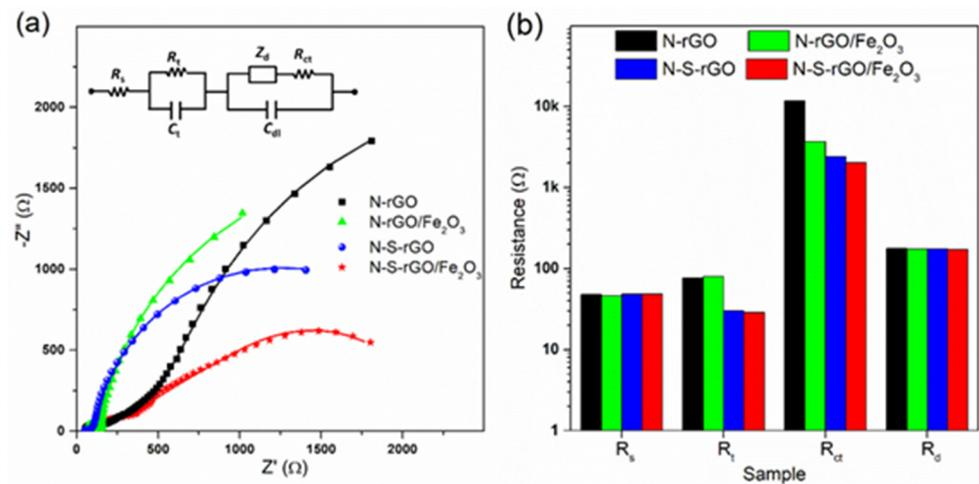
**Figure 9.** The results of the EIS measurements on different samples in a 0.1 M KOH solution: (a) Nyquist plots acquired at a 2500 RPM rotation speed and a 0.68 V potential (the points represent the experimental data, while the continuous lines are calculated from a fitting procedure using the equivalent circuit shown in the inset); (b) calculated resistances.
