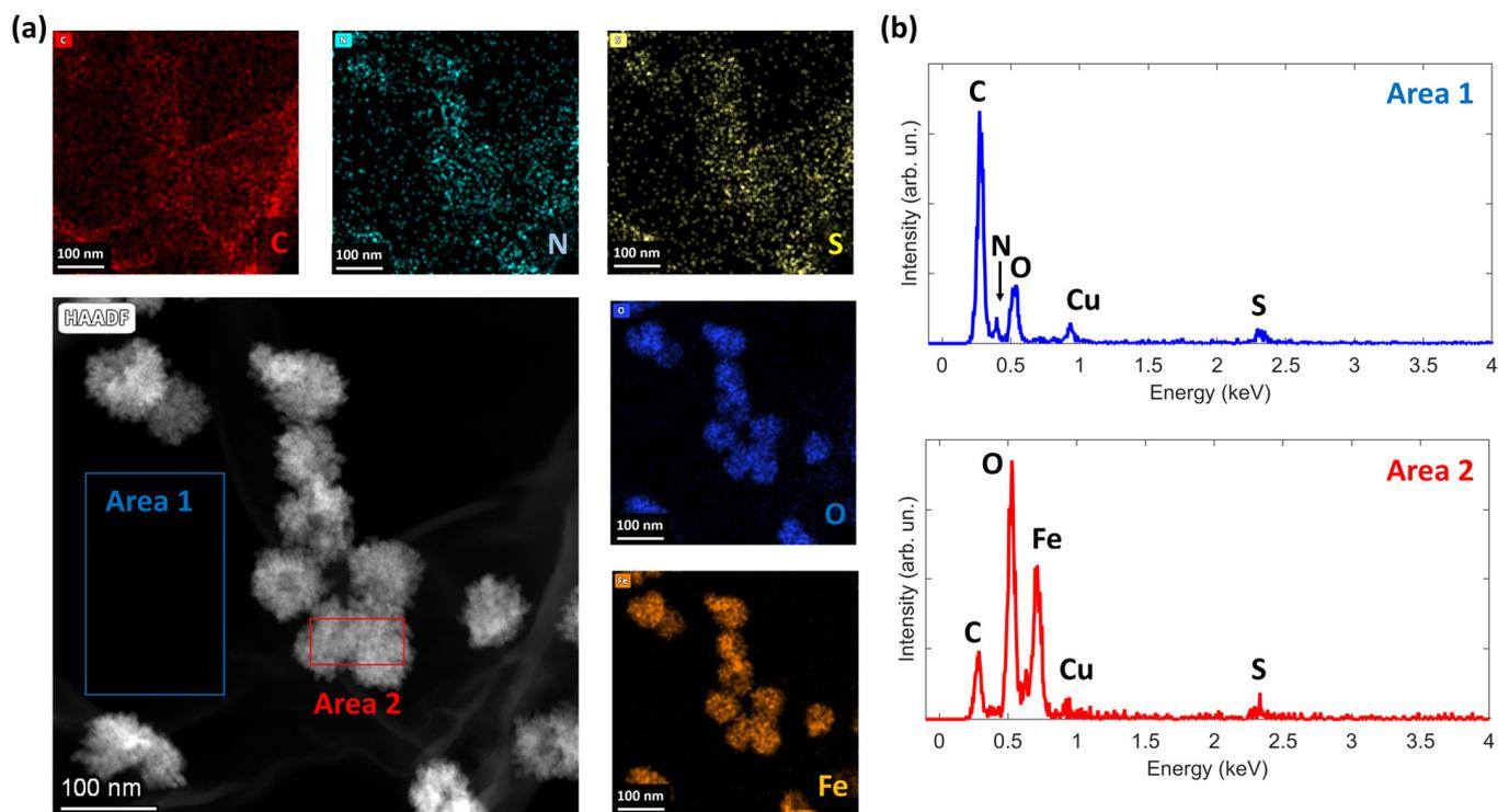
**Figure 3.** EDX analysis of the N-S-rGO/Fe<sub>2</sub>O<sub>3</sub> sample: (a) High-Angle Annular Dark-Field (HAADF) Scanning Transmission Electron Microscopy (STEM) image, alongside corresponding EDX maps for C, N, S, O, and Fe elements; (b) sum EDX spectra obtained from Area 1 (bare rGO flake) and Area 2 (Fe<sub>2</sub>O<sub>3</sub> nanoparticles).
