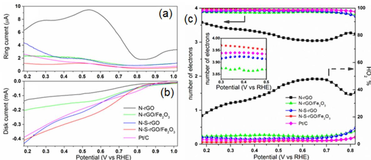
**Figure 8.** Results of RRDE measurements in 0.1 M KOH solution: (a) ring and (b) disk currents measured at 2500 RPM rotation speed; (c) comparison of electron transfer number (left axis) and peroxide percentage (right axis) calculated from curves in (a,b).
