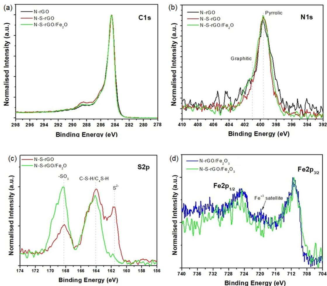
**Figure 5.** XPS HR spectra for (a) C 1s, (b) N 1s, (c) S 2p, and (d) Fe 2p photoelectronic peaks. For the sake of simplicity, in (c), the chemical shift has been reported only for the S 2p<sub>3/2</sub> peak, while S 2p<sub>1/2</sub> can be located 1.18 eV to the left of each S 2p<sub>3/2</sub> peak. In (d), the blue curve refers to data published in Garino et al. [10].
