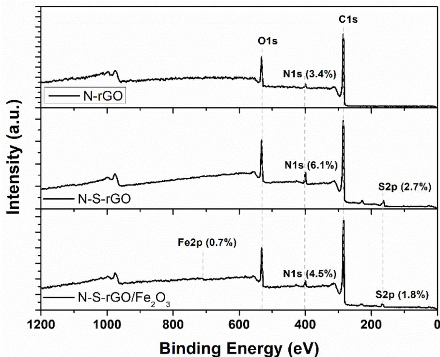
**Figure 4.** XPS survey spectra for N-rGO, N-S-rGO, and N-S-rGO/Fe<sub>2</sub>O<sub>3</sub> samples (dopants' relative atomic concentrations are reported together with Fe amount).
