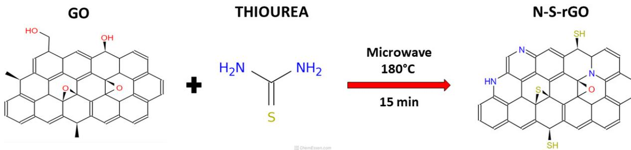
**Figure 1.** Schematic illustration of the synthesis of N-S-co-doped reduced graphene oxide.
