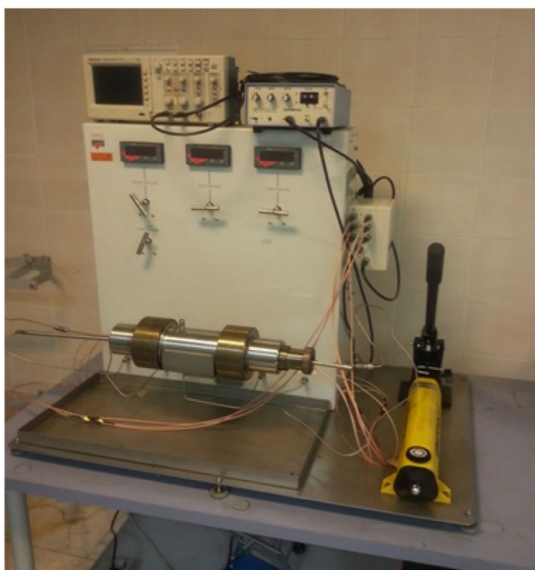
Fig. 1 Experimental and schematic of the acoustic velocity measurement set up
