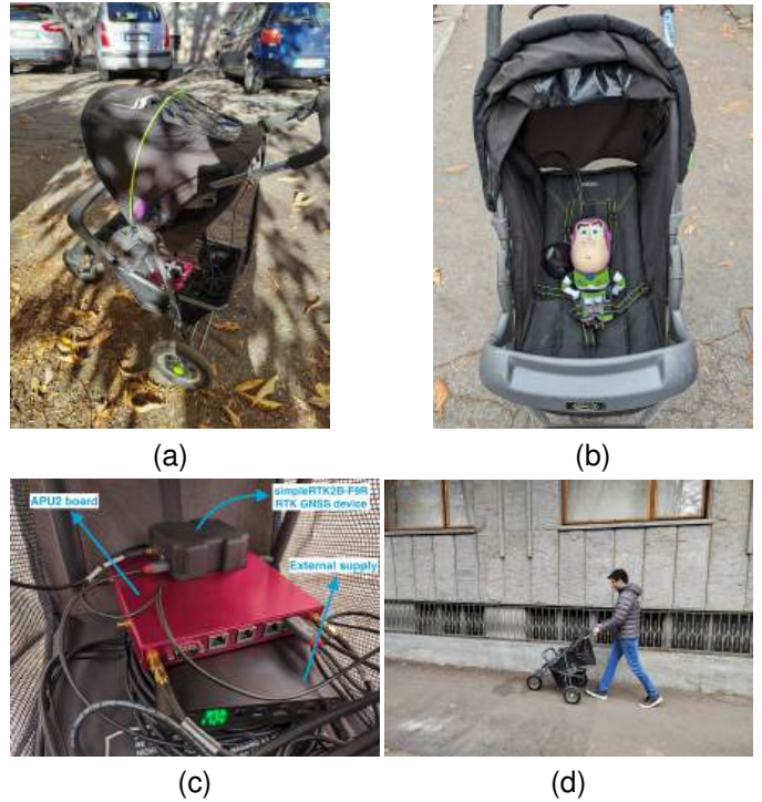
Fig. 3. Field test setup. (a) The equipped stroller, side view. (b) The equipped stroller, front view, with our “VRU” and the DSRC and GNSS antenna. (c) Our hardware boards in the bottom bag of the stroller. (d) A field test example.
