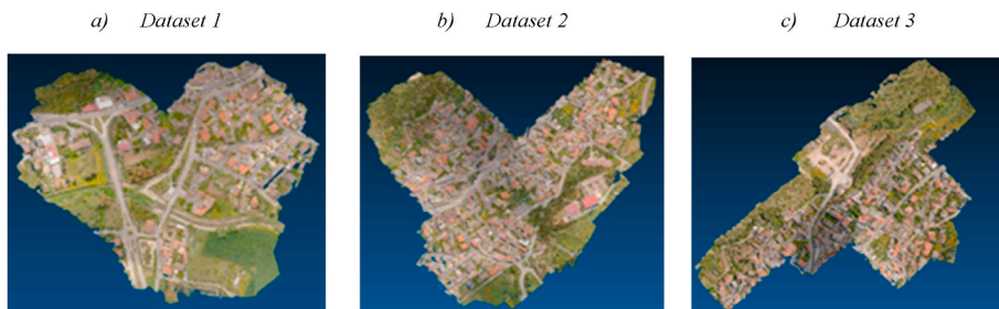
Fig. 2. Photogrammetric point clouds generated on the test areas.
