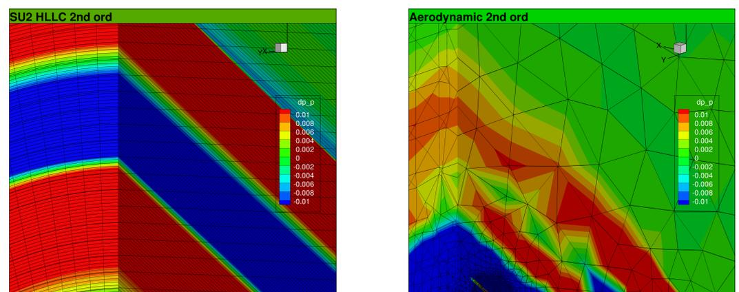
**Figure 7.** CS1 mesh grid, comparison between aeroacoustic (left) and aerodynamic (right) mesh construction approaches.
