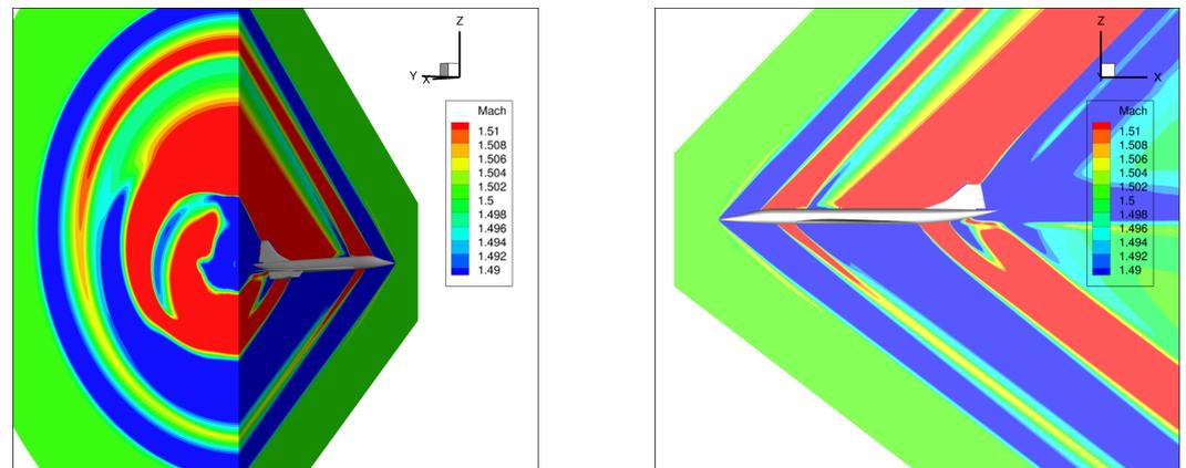
Figure 15. CS1 mach number field for mission point 2, Mach 1.5, AoA 4.5, altitude 15,000 m.
