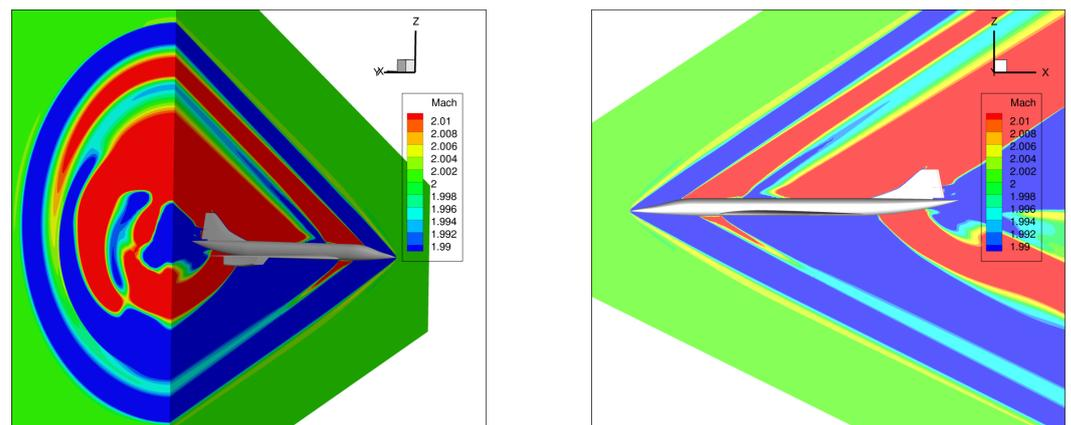
**Figure 18.** CS1 mach number field for mission point 3.
