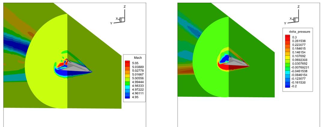
**Figure 21.** CS3 Mach number (left) and delta pressure (right) contours for mission point 6.
