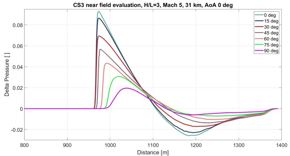
**Figure 22.** CS3 pressure distribution, radial evaluation at  $H/L = 3$ .
