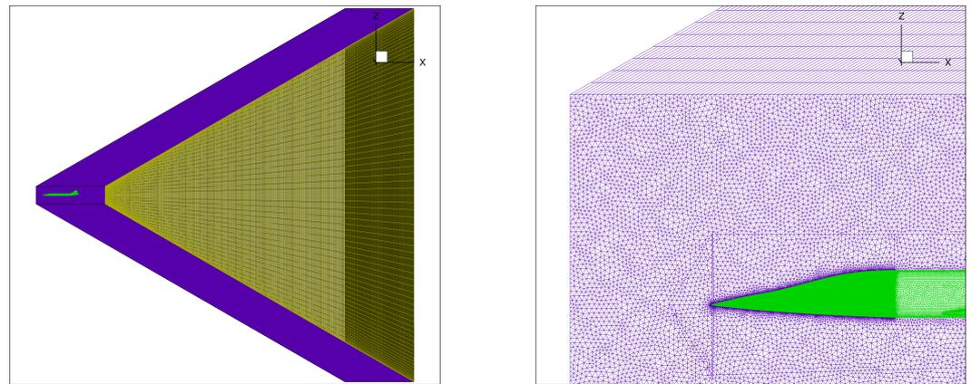
**Figure 6.** CS1 computational grid, overall grid domain (left), and particular cells around the aircraft (right).
