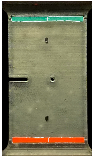
Fig. 4.8 Video frame of specimen type A1 with R = 0.5 mm (nominal) showing the digital recognition of the green (upper) and red (lower) markers. Each cross represents a marker barycentre (see Appendix B).
