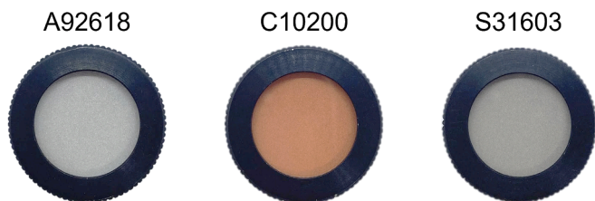
Fig. 2. Cuvettes filled with metal powders for UV-Vis-NIR analysis.
