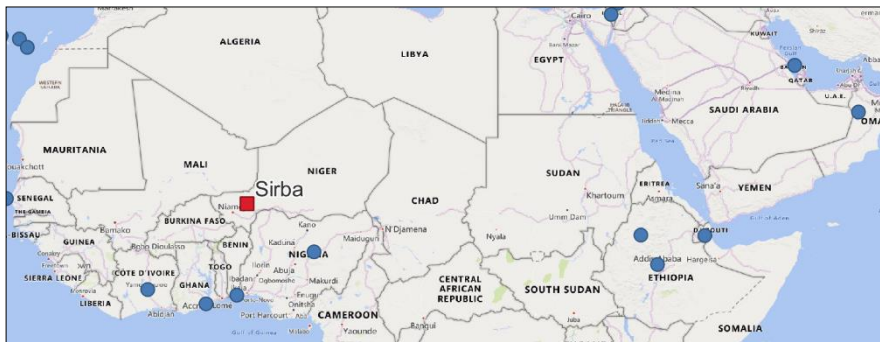
Fig. 1. CORS in north Africa. The blue dots indicate the stations that provide observations to the International GNSS Service (IGS), while the red square is the study area. Data Source: International GNSS Service (IGS), ( https://www.igs.org/ ).
