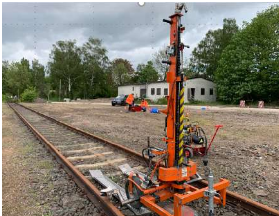
Figure 9: DYNPACT® excitation source used for the measurements.
