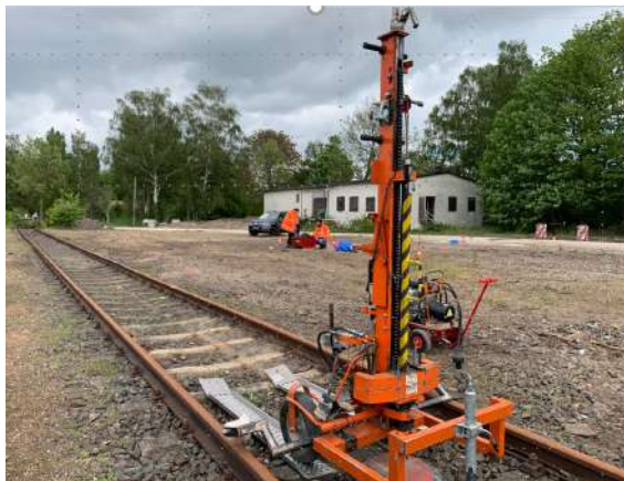
Figure 9: DYNPACT® excitation source used for the measurements.
