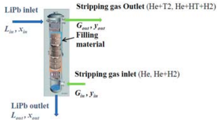
Figure 10. Sketch of the GLC extractor with the nomenclature of the efficiency calculations.
