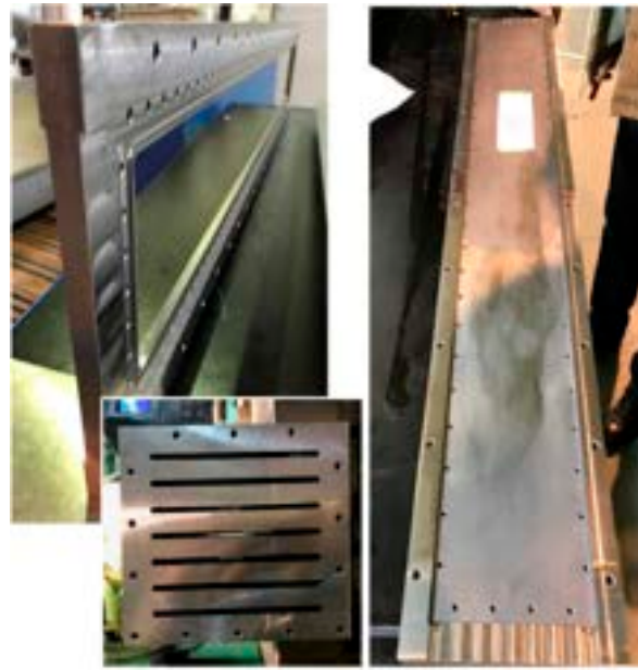
Figure 8. Modular PAV prototype made of vanadium.
