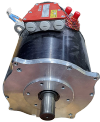
Fig. 2: The BRUSA HSM1-6.17.12 machine under test.
