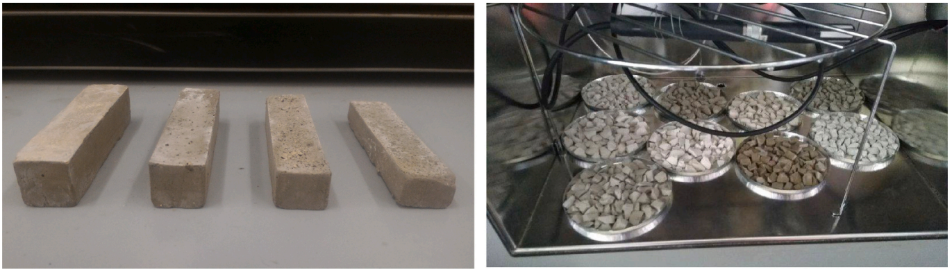
Fig. 1. Samples of CAC-s-1s as obtained from the mold (left) and various cement samples in pelletized form during the testing in a climatic chamber (right).
