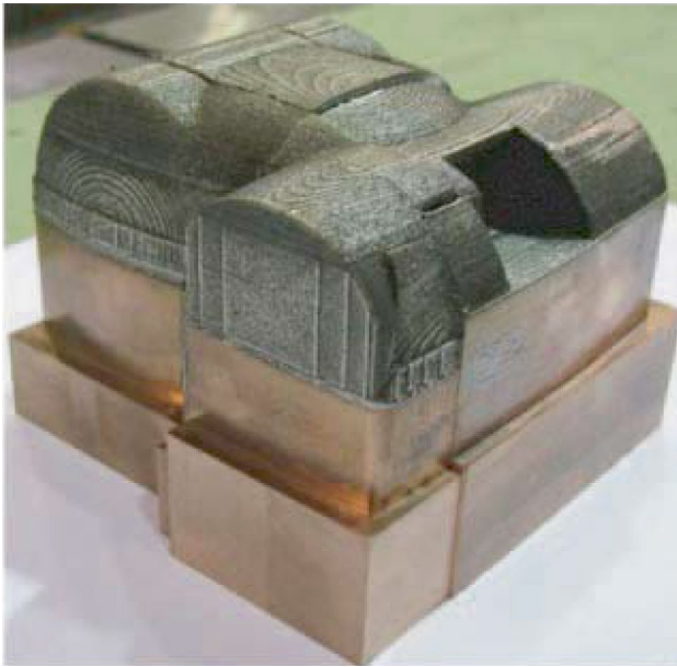
Fig. 19 Functionally graded thermal management mould [159]
