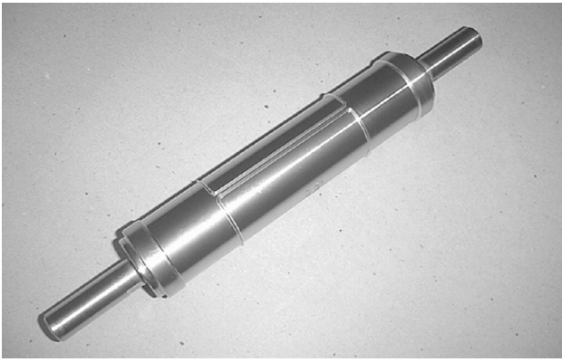
Fig. 32 LP-DED CPM-9 V rotatory cutting die after finishing operation [205]
