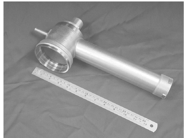
Fig. 31 LP-DED integrated boom/housing [203]
