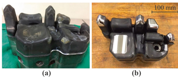
Fig. 11 a Damaged and b restored automotive die [92]
