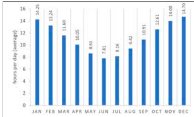
Figure 2. Ex-post installation's average daily switch-on hours for each month.
