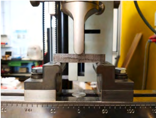
Fig. 3. Mechanical bending test used for proposed SMC materials.
