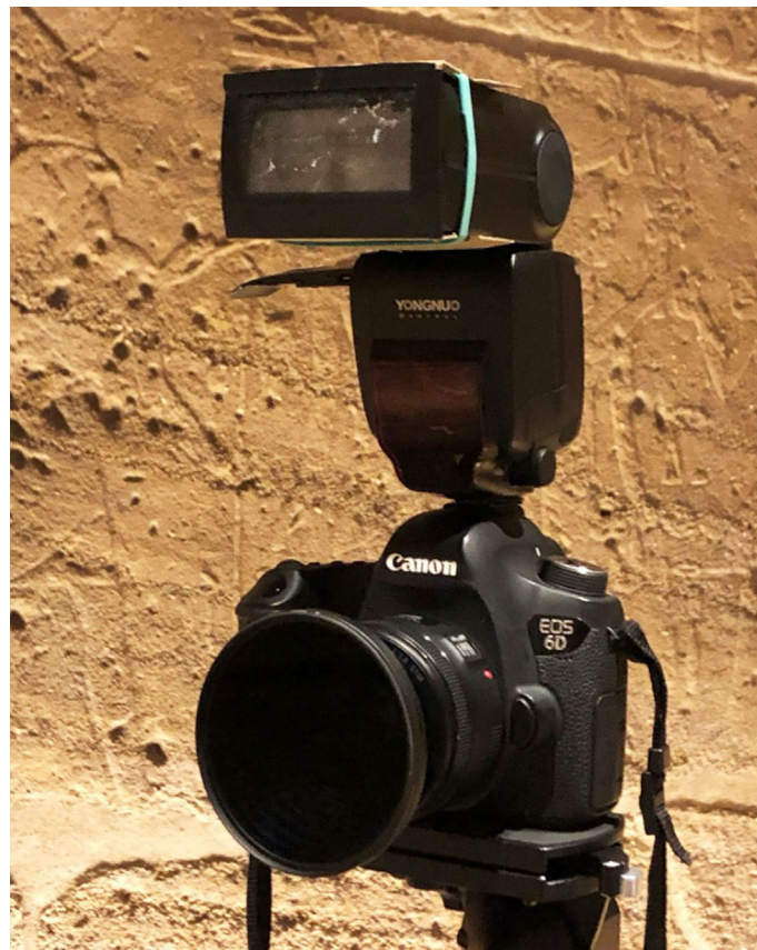
Figure 3. Polarization filters on both camera and flash.
