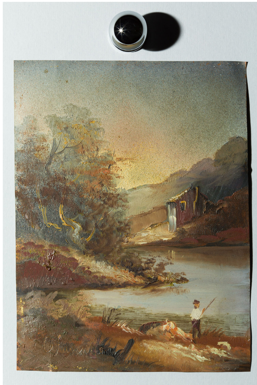
Figure 1. Image of the small painting on copper used as test artifact, with reflective black sphere.
