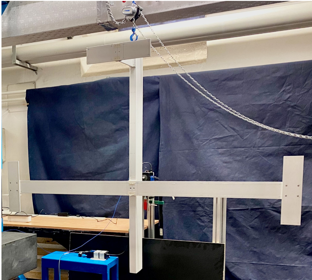
FIGURE 1 Garteur laboratory-scale model and fibre-optic arrangement in the test configuration. The shaker is connected to the rear part of the fuselage, and the suspension system is located in the upper part.
