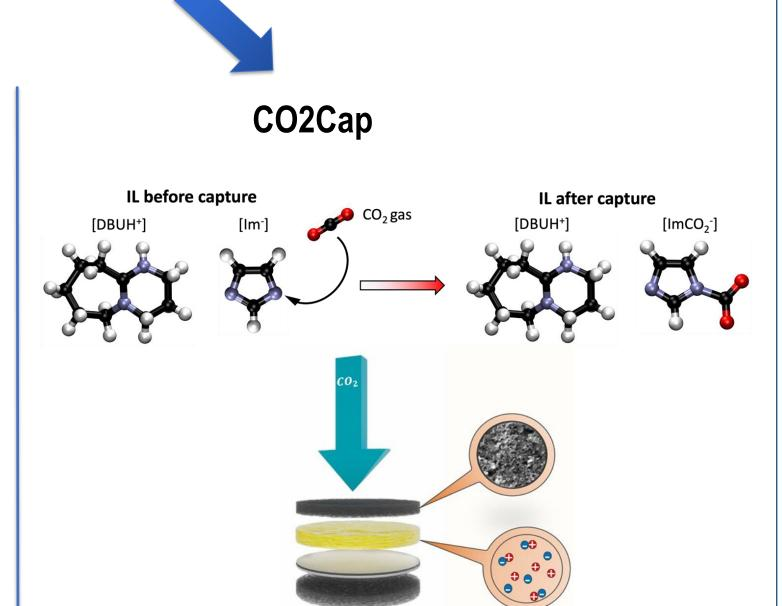
The reaction between the ionic liquid and CO<sub>2</sub> happens only on one electrode, producing a junction across which a voltage difference is created
