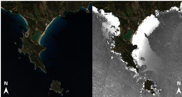
Figure 3. Comparison of uncorrected image (left) with corrected image (right) via WCC with band blue and green.
