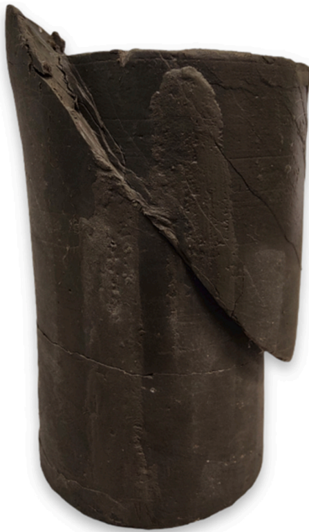
Fig. 6. Typical single well-defined slip surface forming at failure in either monotonic or cyclic triaxial tests.
