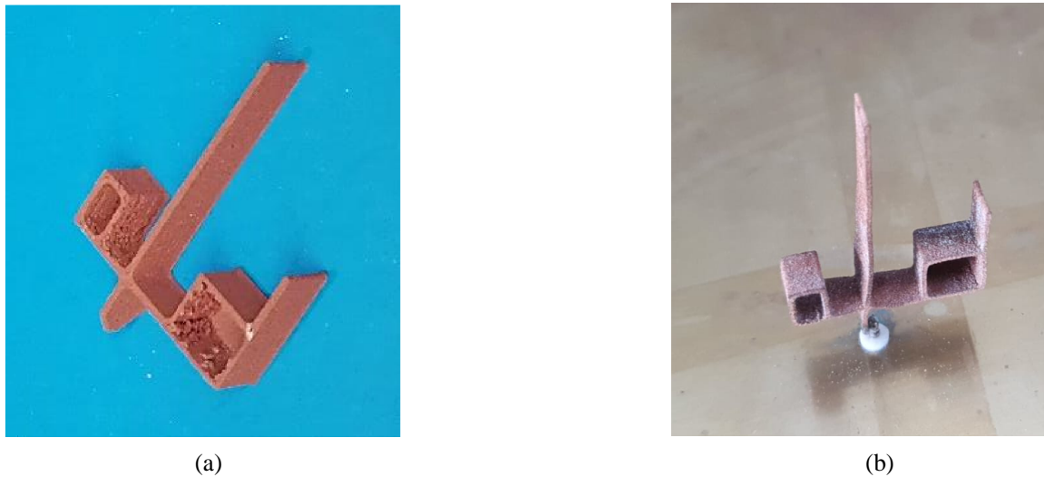
Figure 3. Manufactured antenna. (a) Composite material. (b) Sintered.
