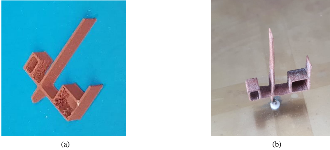
Figure 3. Manufactured antenna. (a) Composite material. (b) Sintered.
