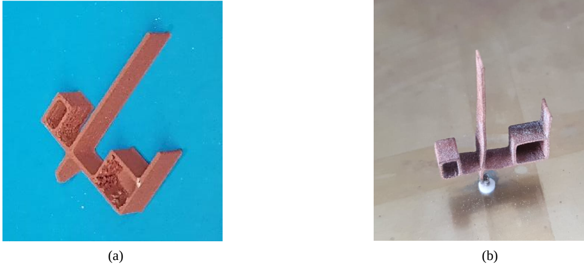
Figure 3. Manufactured antenna. (a) Composite material. (b) Sintered.
