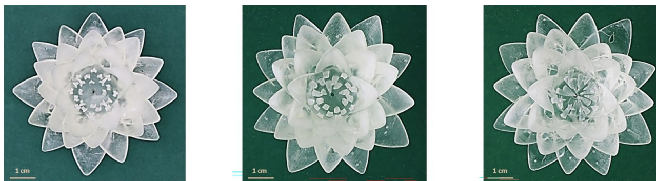
Fig. 8 3D-printed flower structures from formulations Form-IsA-DoDO A (left), Form-IsA-DoDO A:I 1:1 (middle) and Form-IsA-DoDO I (right)
