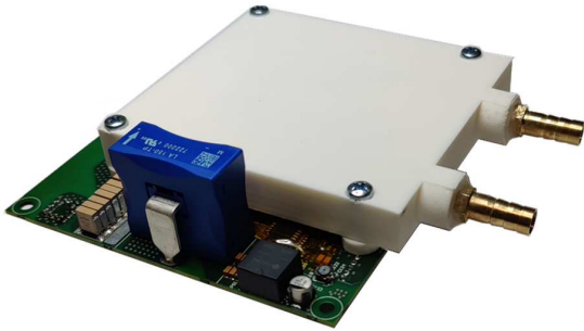
Fig. 4. Bi-component heatsink mounted on the target GaN inverter leg.
