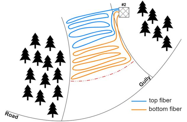
Fig. 8. Two-fiber detection system setup showing the top (blue) and the bottom (orange) fiber.
