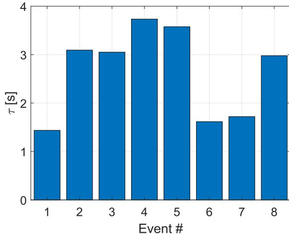
Fig. 10. Bar plot showing on the  $y$ -axis the delays computed by means of cross-correlation in between the SOPAS traces acquired on the two fibers. The related events are identified just as numbers on the  $x$ -axis.
