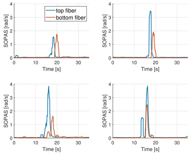
Fig. 9. SOPAS measured during four different launches in the two-fiber configuration.
