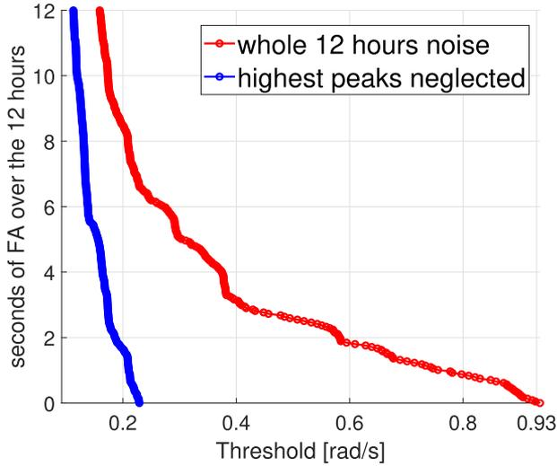
Fig. 7. Seconds of FA over the 12 hours SOPAS acquisition as a function of the threshold value. The red curve has been obtained considering the whole 80 m fiber overnight acquisition, the blue one has been obtained neglecting the two highest spurious spikes.
