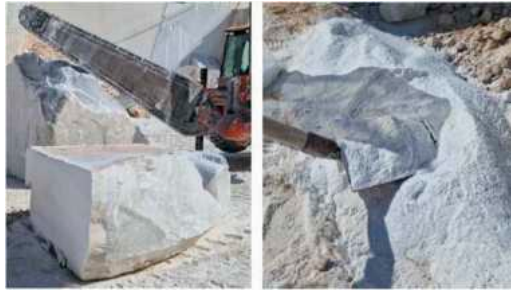
Figure 2. Chain cutting machine used for splitting the marble blocks in slabs (on the left) and the marble sludge obtained during this cutting operation (on the right).
