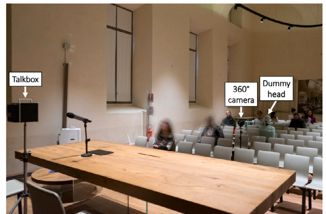
Fig. 4. Picture of the video recording procedure in case of the 360° camera placed in the listening location closest to the target speaker represented by the Talkbox, and one-talker noise at 180° azimuth represented by the dummy head.
