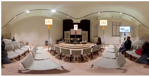
Fig. 5. Equirectangular preview of the visual scene with the listener closer to the target speaker (T) represented by the Talkbox in the front and the one-talker noise at 120° azimuth ( N_{120^\circ} ) represented by the dummy-head.
