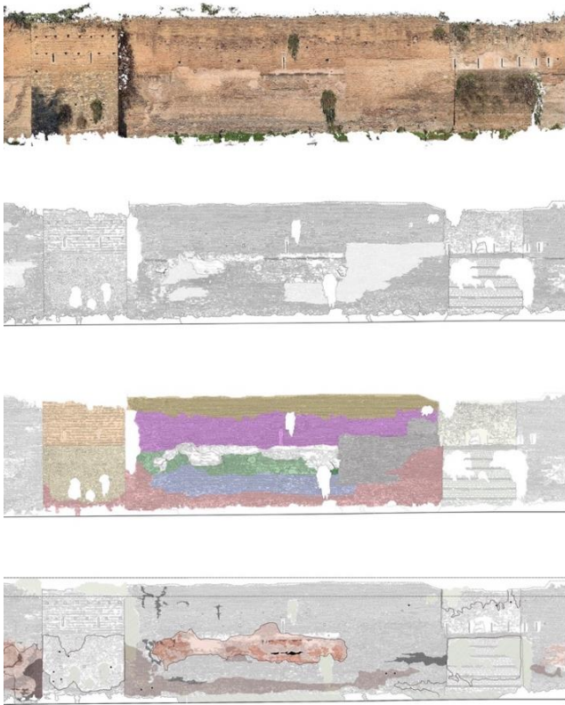
Figure 1. Direct documentation and representation of the Aurelian Walls of Rome, Towers L39-40: from the photogrammetry to the degradation analysis.
