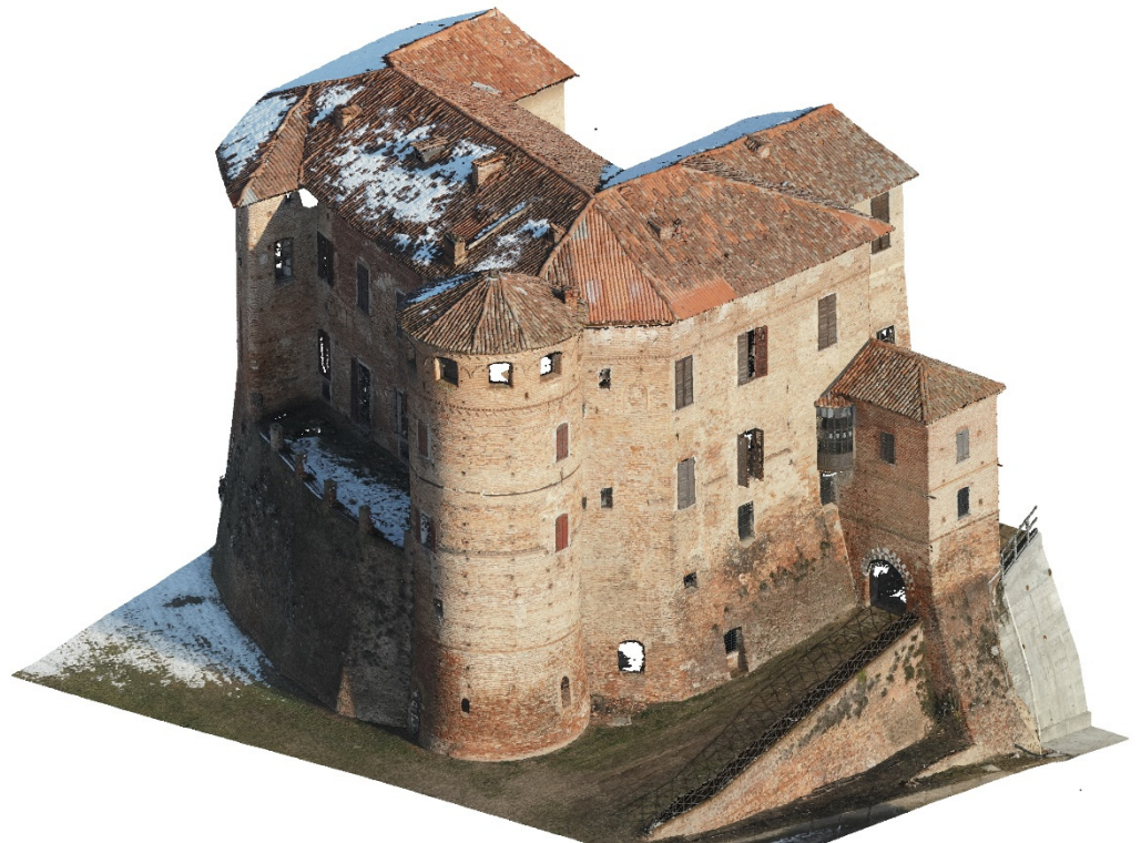
Figure 20. The photogrammetric point cloud acquired by the DJI P1 camera.
