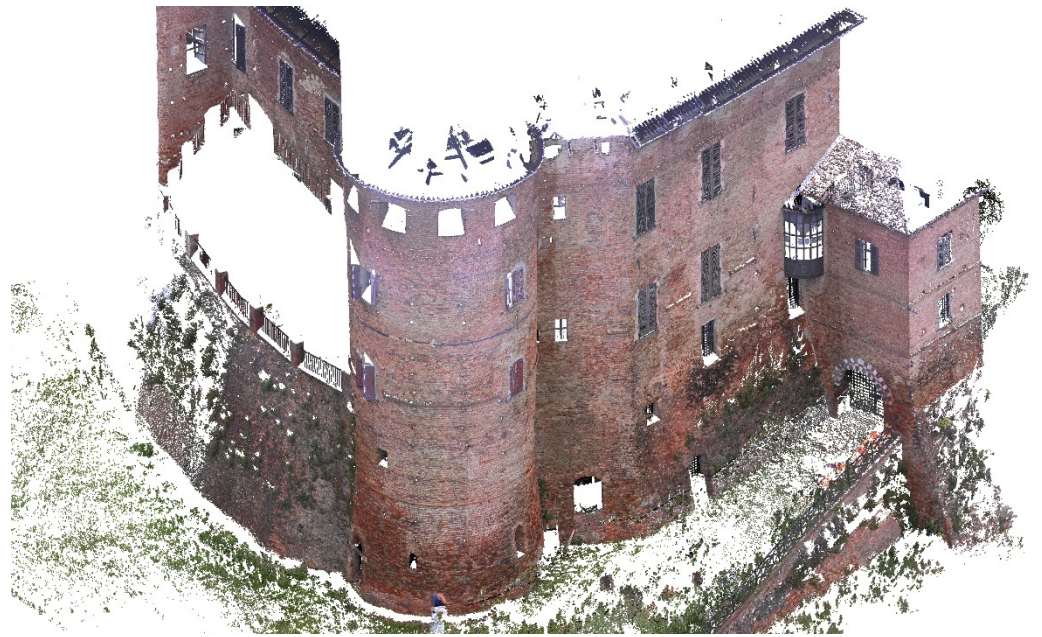
Figure 19. Fused point clouds related to different scans.
