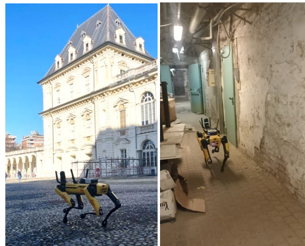
Figure 2. Leica BLK ARC mounted on Spot®, during the data acquisition at the Valentino Castle
