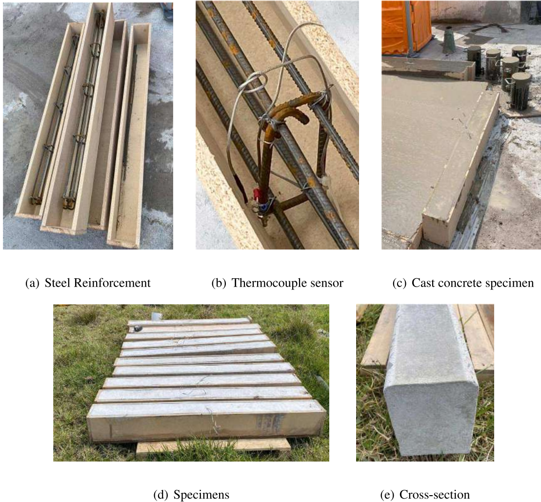
Fig. 1. Specimen fabrication process.
