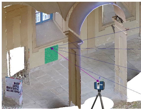
Figure 6. The setup of the 3D points spacing analysis
