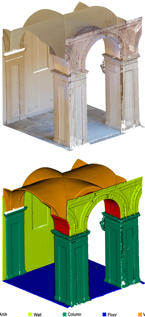
Figure 4. RGB (above) and segmented (below) point cloud for the cloister module of Royal Palace in Turin.
