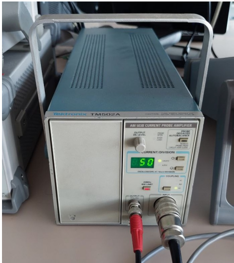
Figure 10: Current Probe Amplifier used to measure the energy consumption
