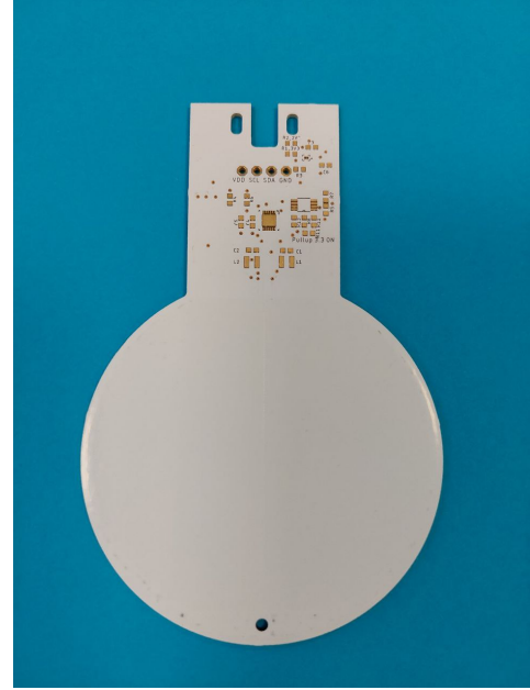
Figure 5: Final PCB with solder mask, modified from [11]
