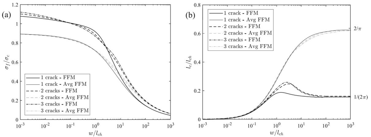
**Fig. 7** Strength estimations  $\sigma_f/\sigma_c$  **a** and critical crack advancements  $l_c/l_{ch}$  **b** provided by FFM (thick curves) and avg-FFM (thin curves) for single, double and triple cracked configurations
