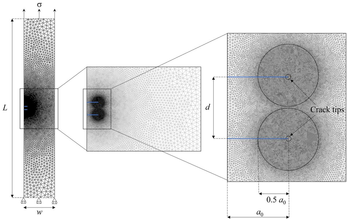
**Fig. 4** Finite element model for the geometry presenting two interacting cracks. The model refers to symmetric crack propagation. It is assumed that  $a_0=d=0.1 w$ , coherently with experimental data
