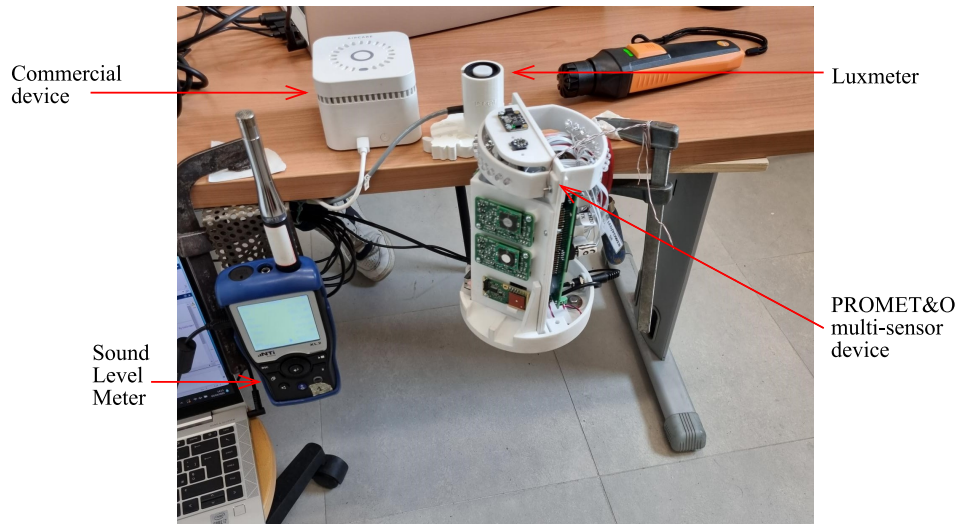
Figure 12. Experimental setup with the PROMET&O multi-sensor, a commercial device, and some reference instruments in an office.
