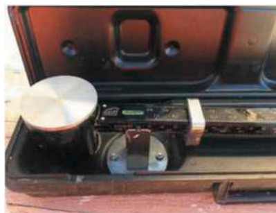
Figure 3. Mud balance used for the unit weight assessment. (Todaro et al., 2023).
