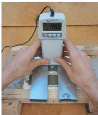
Figure 6. Dynamometer used for the surface compression strength assessment during the test. Todaro et al. (2020).
