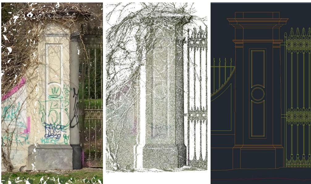
Fig. 6- Detailed elevation view of the study area: mesh from photogrammetric point cloud, laser scanner point cloud, vector drawing (Elaboration: G. Malavasi, F. Natta)
