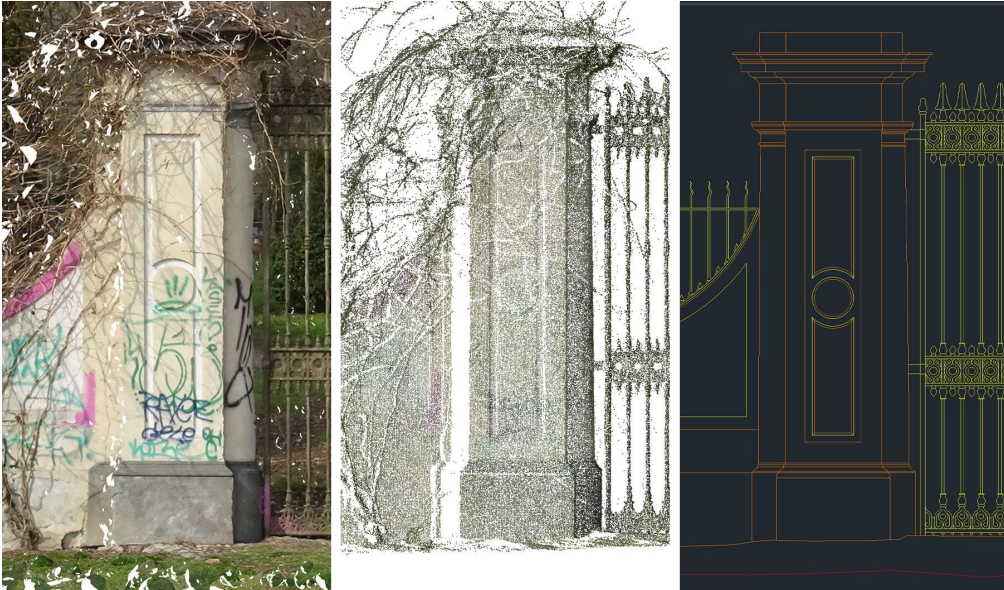
Fig. 6- Detailed elevation view of the study area: mesh from photogrammetric point cloud, laser scanner point cloud, vector drawing (Elaboration: G. Malavasi, F. Natta)
